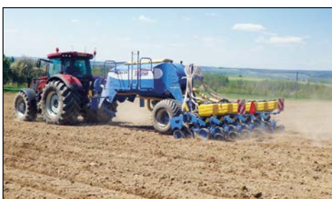
Mounted seed drill for sowing wide-row crops.
