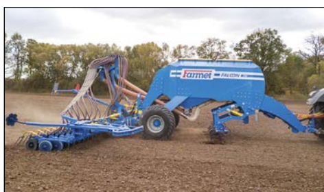
Wide seeding bar for sowing narrow row-drilled crops.
