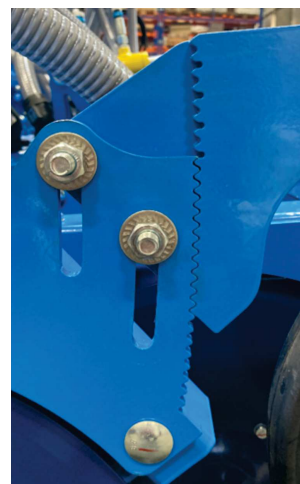
Depth of sowing coulter by 4 cm.
