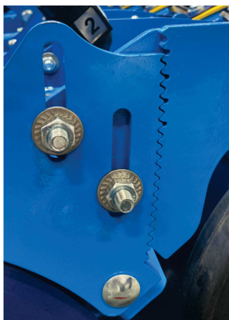
Depth of sowing coulter by 1 cm.
