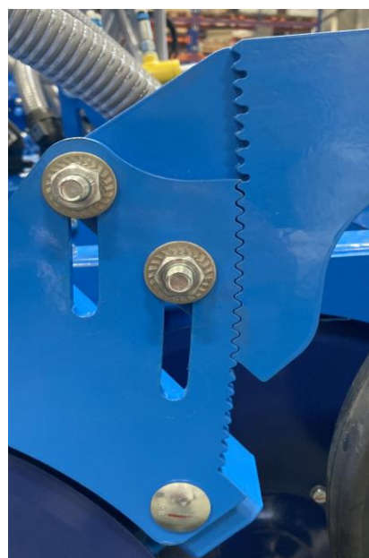
Depth of sowing coulter by 4 cm
