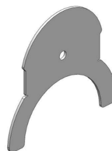
Picture 33 Gauge for assessing the wear of K80
