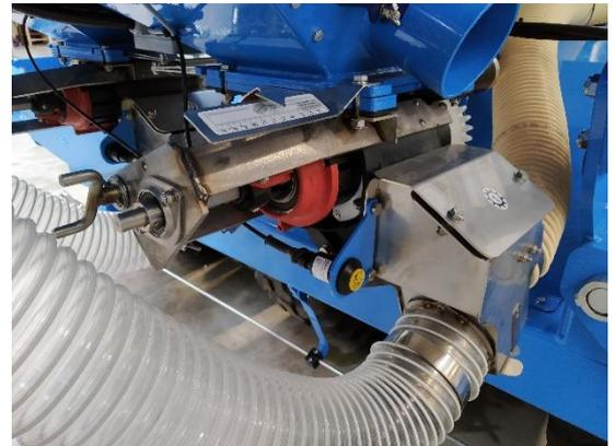
The first step is to set the turnstile according to the calibration table.
