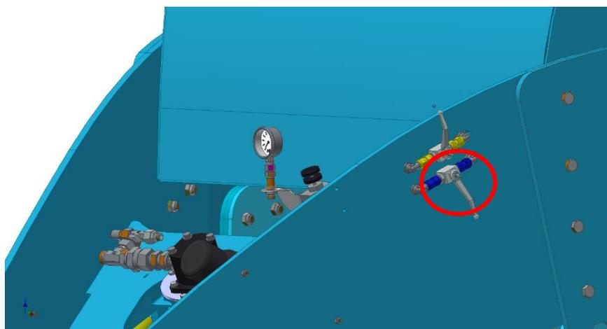
6. Secure the front section for transport, either mechanically or hydraulically (according to the equipment)
