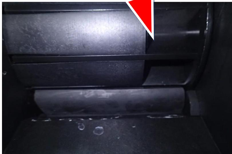
When you empty the container, we recommend “sowing” a few metres with the empty machine and running fan in order to remove the residues of seeds from the feeder and the whole system of the machine.
