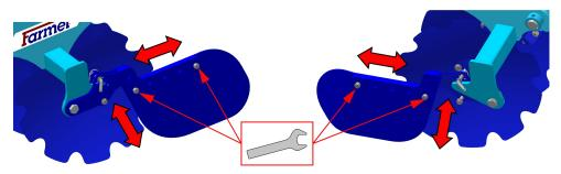
• The position of the edge discs is adjustable and they allow different recess against other discs. The adjustment is executed so that the working depth of the edge discs is lower (approx  $\frac{1}{2}$  -  $\frac{1}{4}$  of the depth of the other discs) so that no unevenness is created on the land.
