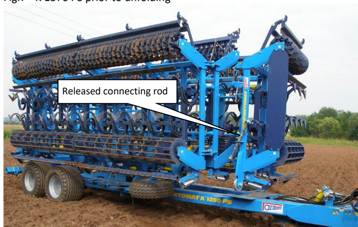
Fig.7 - K 1570 PS prior to unfolding
