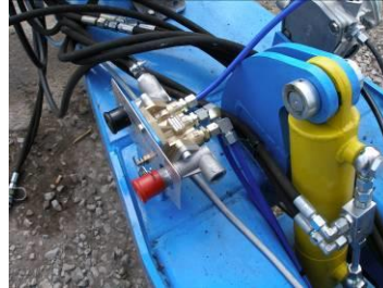
Fig.26 – Hand brake valve control
