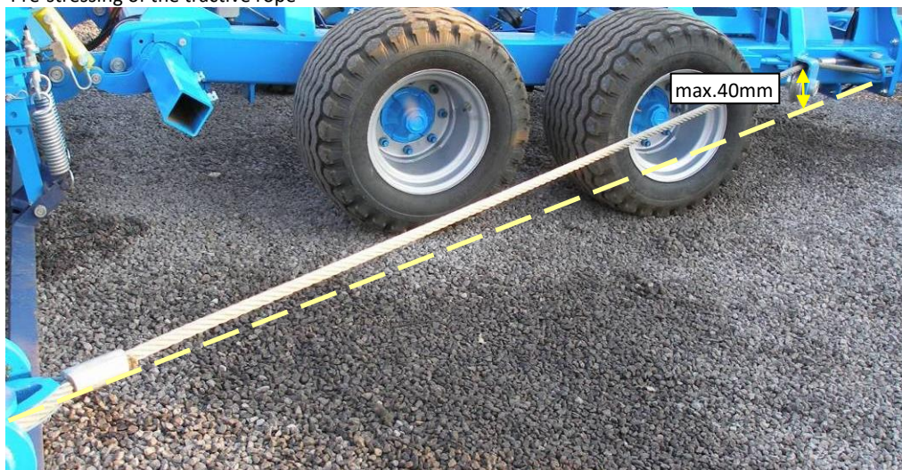
Fig.24 – Pre-stressing of the tractive rope
