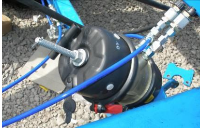
Fig. 28 – Detail of the brake valve control description
