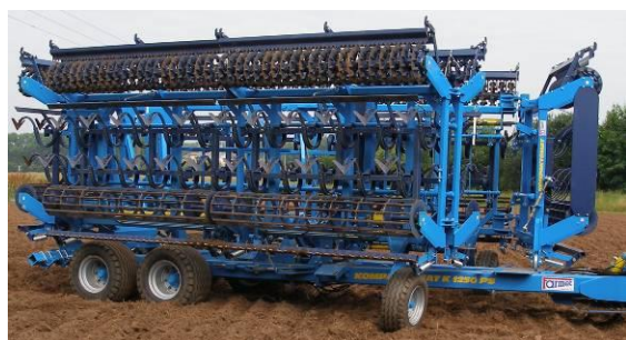
Fig. 30 – Transport position for ploughshare section replacement
