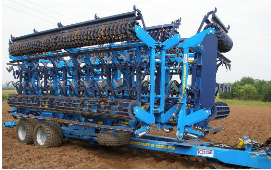
Fig.9 – Auxiliary wheels are in the transport position
