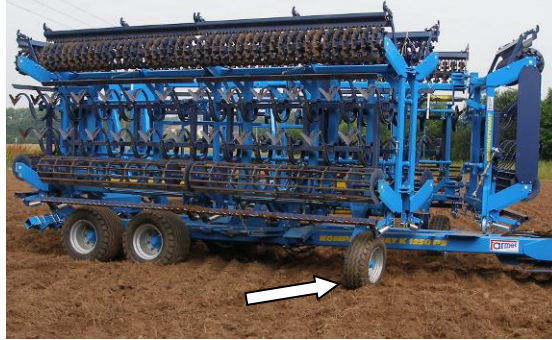
Fig.10 – Auxiliary wheels are prepared for unfolding
