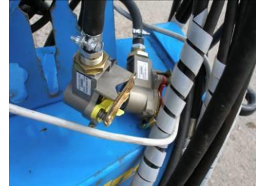
Fig.27 – Quick coupler for brakes
