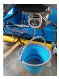
22. Enter the weight into the terminal. For this entry use a window with the name **Acquired value.**
