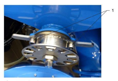
2. Slide out the auger metering unit
