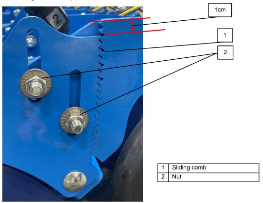
Depth of sowing coulter by 1 cm.
