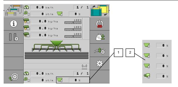
1 Hopper 1 status indicator in % based on sowing test
