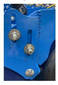
Depth of sowing coulter by 4 cm
