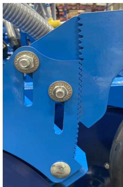
Depth of sowing coulters by 4 cm
