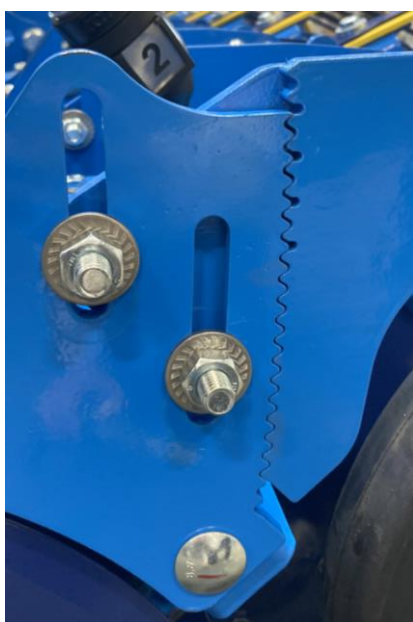
Depth of sowing coulters by 1 cm.
