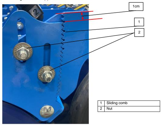
Depth of sowing coulter by 1 cm.
