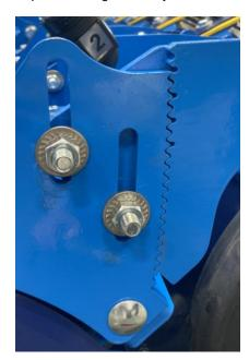
Depth of sowing coulter by 4 cm
