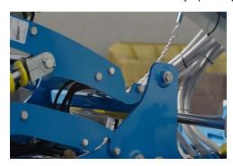
10. Disconnect the quick-release system of the fertilizer hoses and the hose tension chain.
