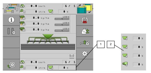
1 Hopper 1 status indicator in % based on sowing test 2 Open menu of real-time values (choose which ones I currently want to display)
