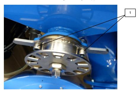
2. Slide out the auger metering unit
