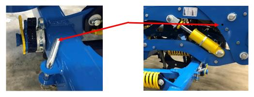
7. Raise the front section by operating the hydraulics from the tractor until the lower link is released.
