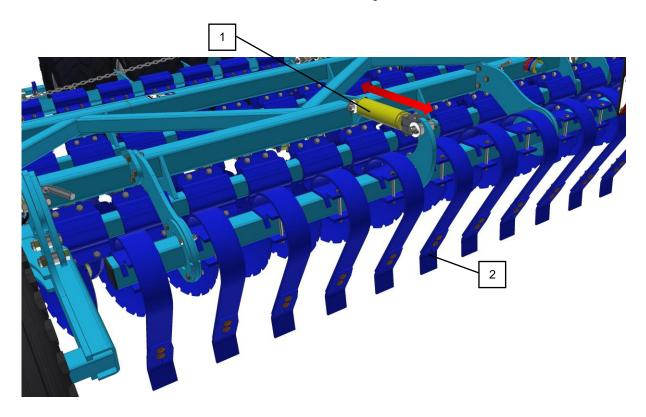
1 Flexi board piston rod 2 Flexi board working body
